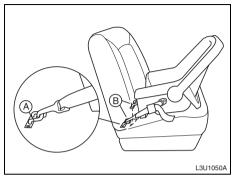
With this type of child restraint, use the LATCH system instead of the vehicle's safety belts to secure the child restraint.
